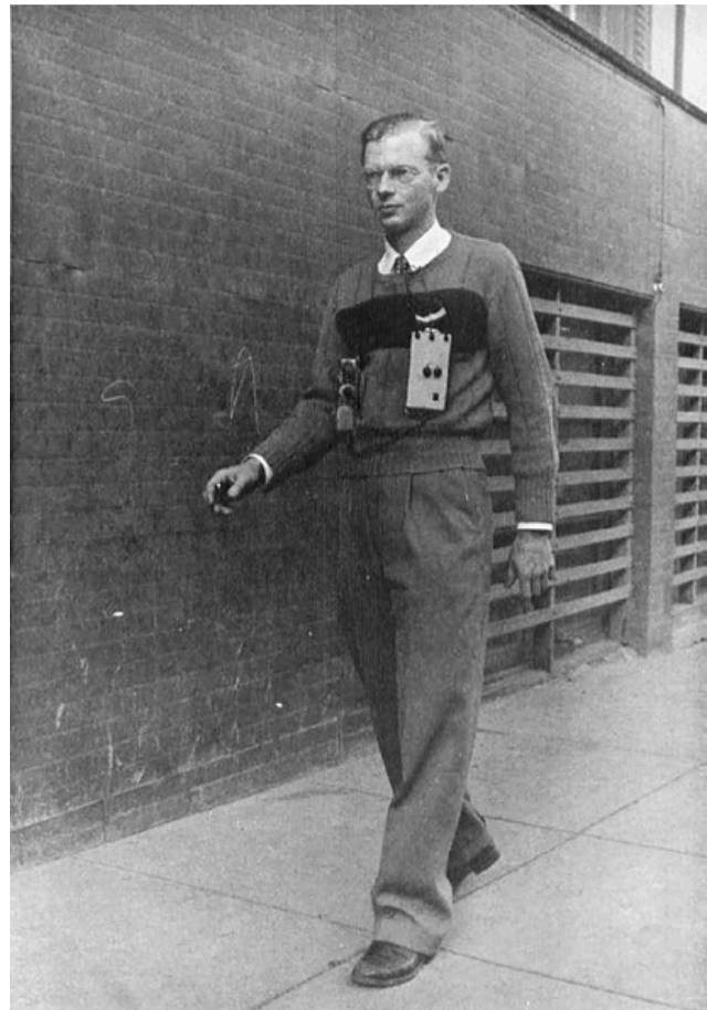
Holter's original wearable health technology: the radioelectrocardiograph, c. 1957. Courtesy of the New York Academy of Sciences.
