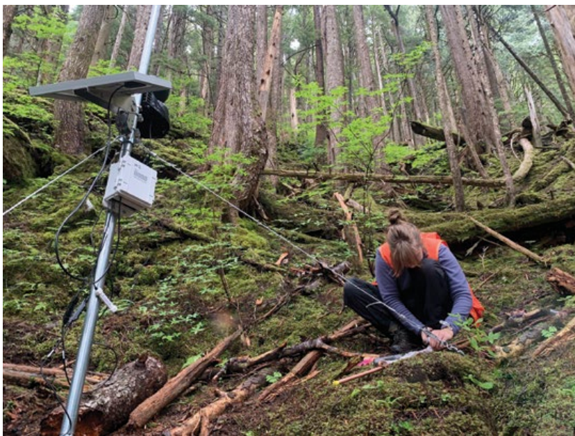
A Sitka Sound Science Center employee helps install an experimental soil moisture monitoring site on a hillslope above Sitka.
